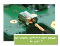
The versatility and flexibility of machined receptacles is further evidenced by the numerous ways they can be used to accomplish various other objectives. For instance, in making board-to-board connections there are multiple receptacle design styles suitable for robust/power applications on .100" pitch or greater, as well as for fine pitch down to .8 mm, for low-level, high-speed signal transmission. In addition, SMT and HSMT options offer added design flexibility, allowing I/O and component
