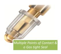
Most importantly, critical applications call for machined pin receptacles because a machined receptacle – fitted with a stamped, multi-finger contact that provides an interface with redundant points of contact and a gas-tight connection – delivers vastly superior performance. These contacts maintain their normal and characteristic forces even after extended exposure to shock, vibration and environmental changes. They will function reliably to a
